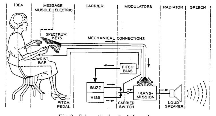
Fig. 8-Schematic circuit of the voder.
